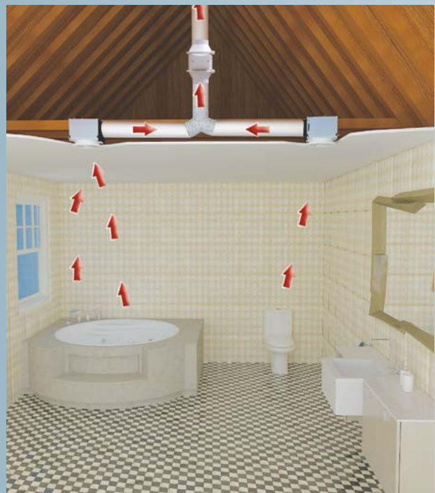
Dual ventilation kit installation
