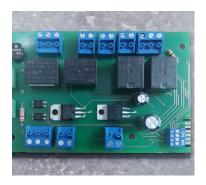
Integrated controller provides automatic switching between supply and exhaust modes in accordance with code requirements. DIP switch of cyclic timer is located on the control board.
