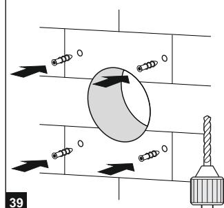
Installation of X star wall-through ventilation fans
