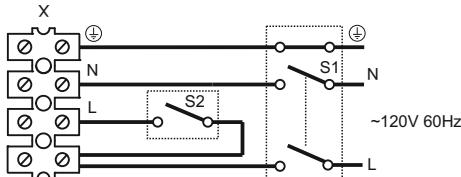
**Electrical connection of ventilation fan with timer or humidity sensor and standard wall switch**
