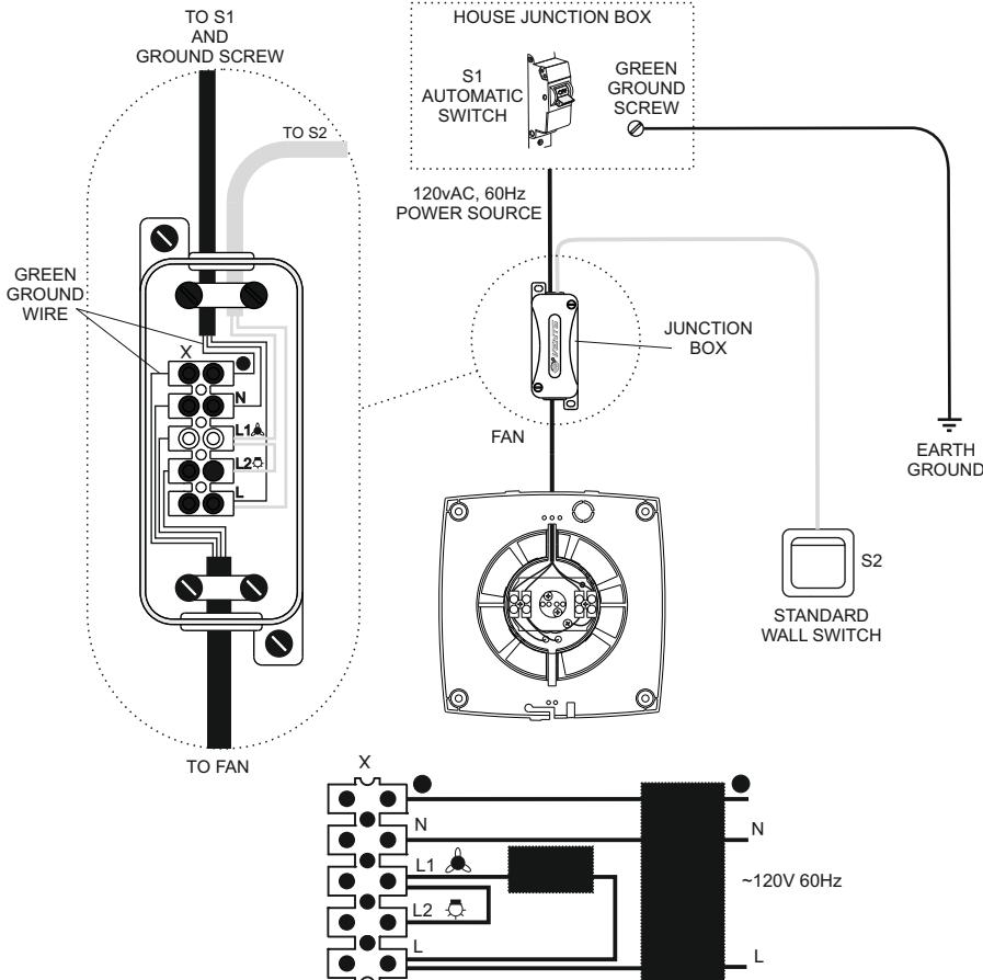
**Electrical connection of Xstar fan and standard wall switch for separate enabling the motor and lamp**
