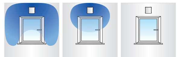
Air flow distribution of depending on different position of the air flow control
