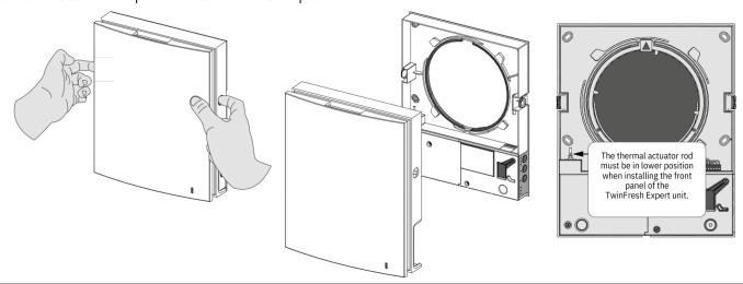
5. Fix the back part of the indoor unit on the wall with the screws supplied with the mounting kit of the ventilator. Remove the two retaining screws from the left transparent cover to enable access to the terminals.
