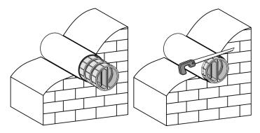
10. Install the outer ventilation hood. For this, see the user's manual for the hood.
