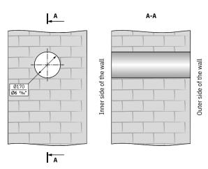
2. Install the air duct in the wall and fix it with mounting foam. The air duct end must protrude for the distance that enables installation of the outer ventilation hood (see the User's manual for the outer ventilation hood).
