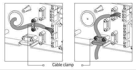
7. Install the cartridge into the air duct as figured below. The pointer must be directed upwards. Then fix the wire with the protruding clamp and connect the socket connector to the circuit board.
