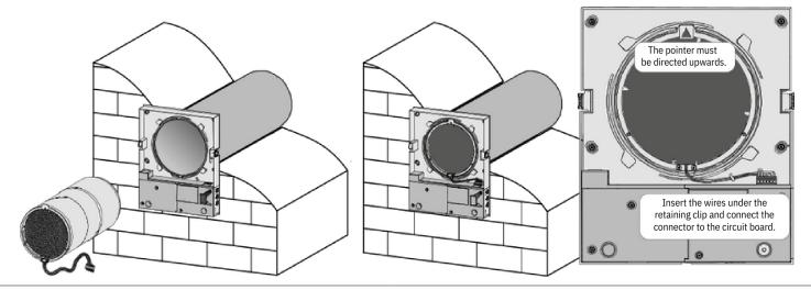
8. Install the front part of the indoor unit. The thermal actuator rod must be in lower position when installing the front panel, as shown in the figure in Section 4 on page 2.
