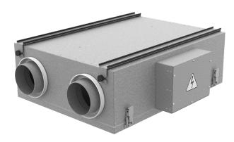
Energy Recovery Ventilators are the complete whole house ventilation system designed to bring a continuous supply of fresh air into the house while exhausting an equal amount of stale air
