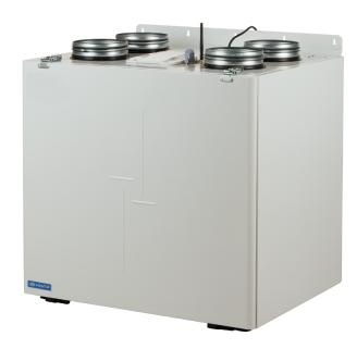
The air-handling units are the fully featured ventilation units with heat recovery for air filtration, fresh air supply and stale air extract. During operation the extract air heat is transferred to the supply air stream by the highly efficient plate heat exchanger
