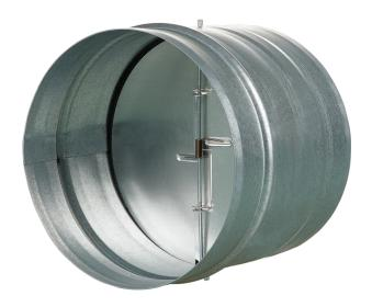
KOM U spring-loaded backdraft damper is manufactured of 24/26 gauge galvanized steel and contains rubber seal, it is especially designed to prevent backdraft. KOM U also prevents the entry of birds and other wildlife
