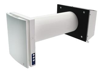
The TwinFresh Expert RW1-85-2 V.2 is a state-of-theart 50 CFM (max) Energy Recovery Ventilator (ERV) designed to provide you with a continuous supply of fresh, filtered air, all the while helping to reduce your energy costs. Wi-Fi enabled, it will provide ventilation for single rooms of up to 500 square feet. Perfect for new builds, renos, apartments, cottages and tiny homes. No ducting required
