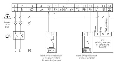
Connection of additional external control contacts is implemented in the control unit. For accessing the control unit open the unit door, release the screws fixing the shielding and remove it.
