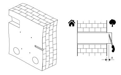
**3.** Fix the mounting template on the wall to install the air ducts.
