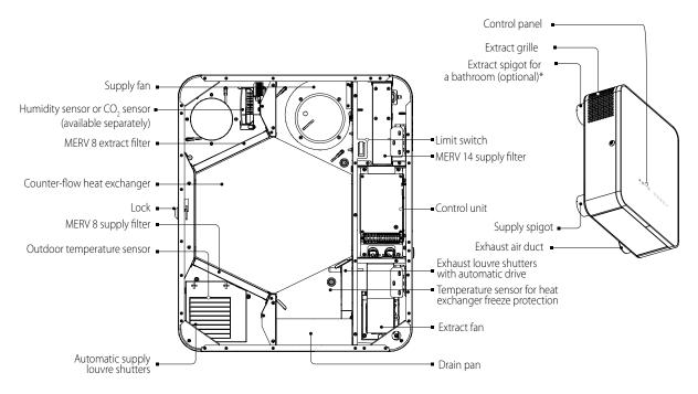
Warm stale extract air from the room flows to the unit, where it is filtered by the extract filter, then air flows through the heat exchanger and is exhausted outside by the extract fan.
