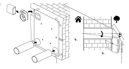
**4.** Fill the spaces between the air ducts and the wall with a mounting foam through the specially designed holes in the mounting template.
